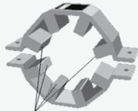
CONCENTRATION DE MEMES POLES ARRANGES RADIALEMENT A L'AXE DU CONDUIT
